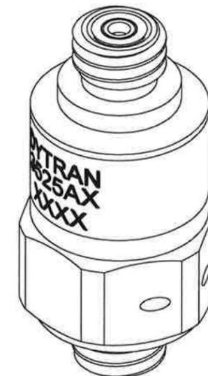
MOUNTING RECOMMENDATIONS: PREPARE MOUNTING SURFACE FLAT TO .001 TIR. TAP 10-32 UNF-2B  $\nabla$  .20 MIN., RECOMMENDED MOUNTING TORQUE 15LB-IN +5/-0 LB-IN. FOR BEST FREQUENCY RESPONSE, MOUNTING SURFACE MUST CONTACT ENTIRE ACCELEROMETER MOUNTING SURFACE.
