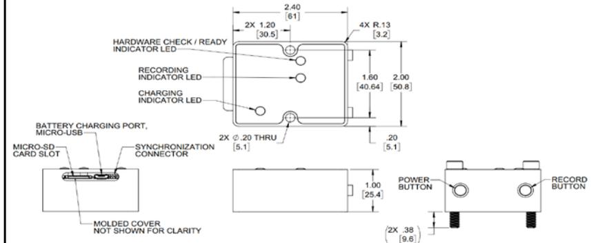
Units on the line drawing are in inches, units in brackets are in millimeters. Refer to 127-4400B for more information.
