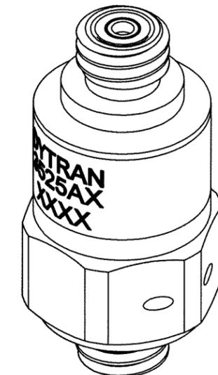
MOUNTING RECOMMENDATIONS: PREPARE MOUNTING SURFACE FLAT TO .001 TIR. TAP 10-32 UNF-2B  $\nabla$  .20 MIN., RECOMMENDED MOUNTING TORQUE 15LB-IN  $\pm$  5/-0 LB-IN. FOR BEST FREQUENCY RESPONSE, MOUNTING SURFACE MUST CONTACT ENTIRE ACCELEROMETER MOUNTING SURFACE.
